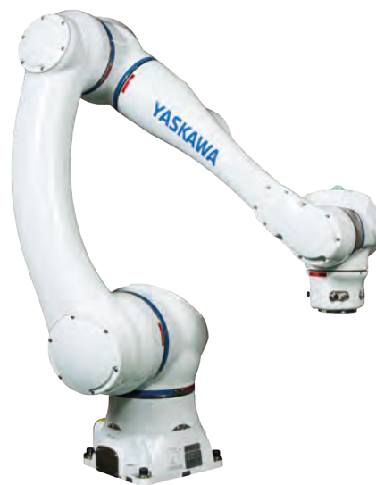
Collaborative robot MOTOMAN-HC20DTP
