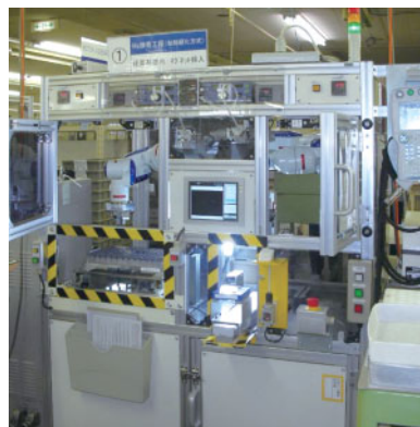
▲ Motor parts assembly device installed at our Tokyo Plant We are installing a device using the SDA5D in the motor fabrication process at our Tokyo Plant to automate the work of motor assembly. This device has an SDA5D with hands for holding motor parts. The device is carrying out assembly work by grasping parts with both hands.
