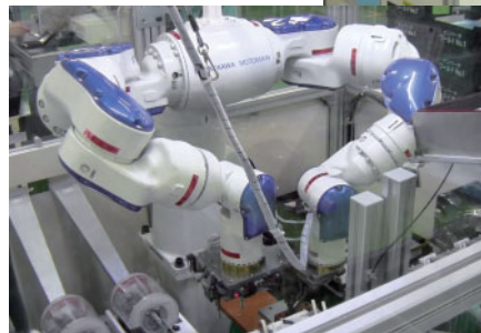
▲ Small parts (cooling fin) assembly device installed at our AC drive plant We are automating small part assembly work by installing equipment that uses the SDA5D at the Drive Center of our Drives Division to work on preparatory processes in the circuit board fabrication process. Parts were formerly put together manually, after which the job of screw tightening would be carried out. We have automated this work, equipping one of the robot's arms with a hand that holds parts and the other with a hand that holds an electric screwdriver. This enables the robot to perform the same work as a person at greater speed.
